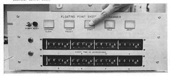
TIME OF ARRIVAL system is used with the shock tube for determining the velocity of shock waves. Dick McAvoy (7335) installs one of the 50 code cards which measure the time it takes shock waves to move between various points along the eight-foot shock tube.
